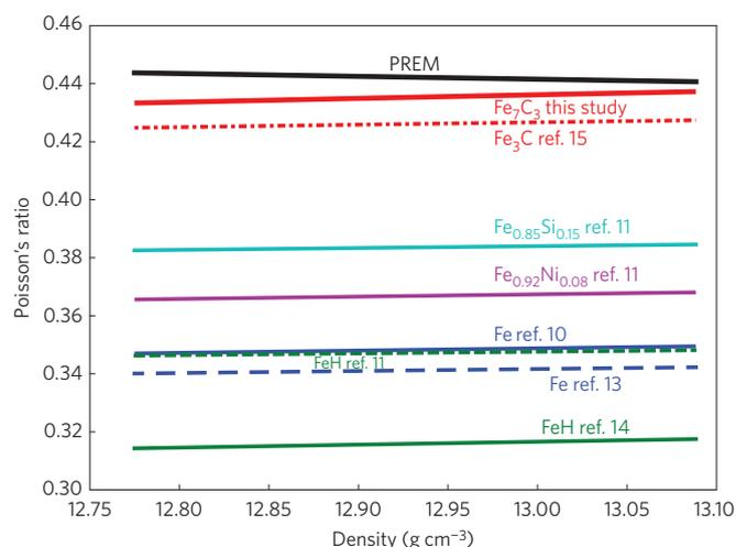
**Figure 4 |** Extrapolation of Poisson's ratio to the densities estimated in the Earth's inner core using Birch's law. The only element which significantly increases the Poisson's ratio of iron is carbon. Moreover, the estimated Poisson's ratio of  $\text{Fe}_7\text{C}_3$  nearly approaches the Poisson's ratio of the preliminary Earth reference model (PREM; ref. 2) at densities near the centre of the inner core.
