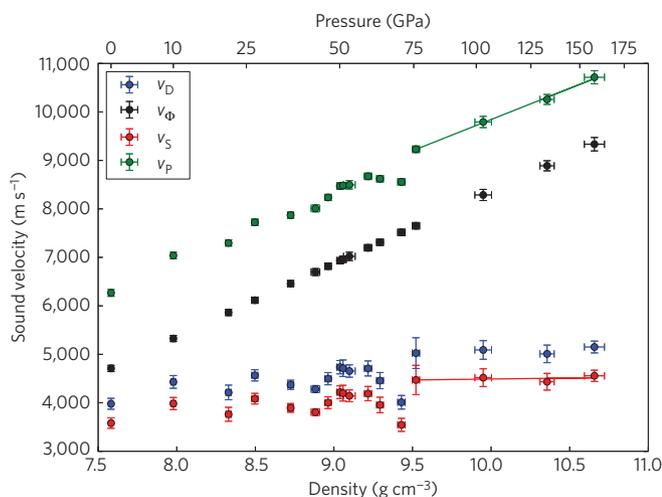
**Figure 3 |** Variation of Debye sound velocity  $v_D$ , bulk sound velocity  $v_\phi$ , shear wave velocity  $v_S$  and compressional wave velocity  $v_P$  of  $\text{Fe}_7\text{C}_3$  with density. Linear fits to the non-magnetic data for compressional (green) and shear wave (red) velocities were used to extrapolate sound wave velocities and Poisson's ratios to conditions of the Earth's inner core.
