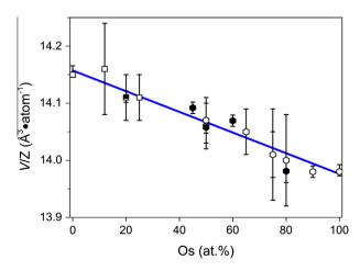
**Fig. 4.** Concentration dependence of atomic volumes of Ir–Os alloys and corresponding linear fit. Squares and hexagons correspond to *fcc* and *hcp* alloys respectively. Literature values [22,28,29] are shown as open symbols and filled symbols are for the values obtained in the current study.
