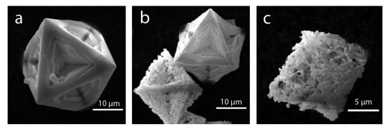
Fig. 3. SEM images of (NH<sub>4</sub>)<sub>2</sub>[Ir<sub>0.65</sub>Os<sub>0.35</sub>Cl<sub>6</sub>] precursor (a) and its decomposition product (b and c).
