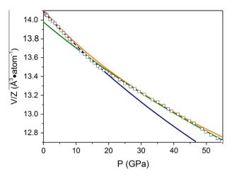
**Fig. 7.** Pressure dependence of atomic volume for *fcc*-Ir<sub>0.80</sub>Os<sub>0.20</sub> sample. Lines show the second-order BM-EoS fits for the whole pressure interval (orange), below 20 GPa (blue) and above 20 GPa (green). (For interpretation of the references to colour in this figure legend, the reader is referred to the web version of this article.)
