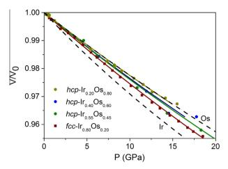
Fig. 5. Relative volume compressions for Ir [4], Os [7] (dashed lines), and Ir-Os alloys (solid lines).
