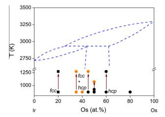
**Fig. 1.** Experimental Ir–Os binary phase diagram [15]. Squares and hexagons correspond to *fcc* and *hcp* alloys synthesized in the current work; two-phase samples are shown by circles; arrows indicate transformations upon heating.
