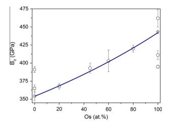
**Fig. 6.** A composition dependence of bulk moduli for pure Ir, Os and Ir–Os alloys. Line corresponds to  $B_0(x_{Os})$  dependence according to Eq. (2) with fixed  $B_0$  = 354 GPa for Ir [4] and fitted  $B_0$  for Os (fitting gives  $B_0$  = 442 (2)). Star shows bulk modulus for diamond [39].
