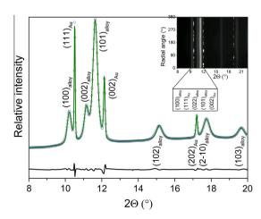
**Fig. 2.** Least-square fit for hcp-Ir<sub>0.20</sub>Os<sub>0.80</sub> with gold as internal standard at 28.6 (5) GPa ( $\lambda$  = 0.4145 Å). Experimental data-points are shown as circles, refined profile – as solid line, difference curve is shown at the bottom. Inset shows radial sweep of 2D image.
